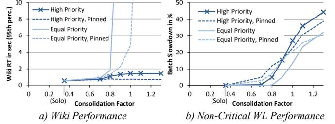
Figure 5. Pinning VCPUs of Critical Workloads (Scenario B)
