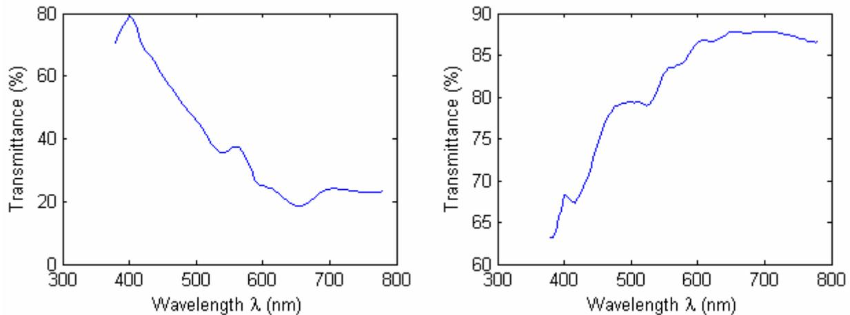
Figure 3. Left: percent spectral transmittance of the cooling filter. Right: percent spectral transmittance of the warming filter.
