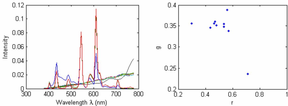
Figure 2. Spectral power distributions of the illuminants (left) and plot of  $r$  vs.  $g$  values.
