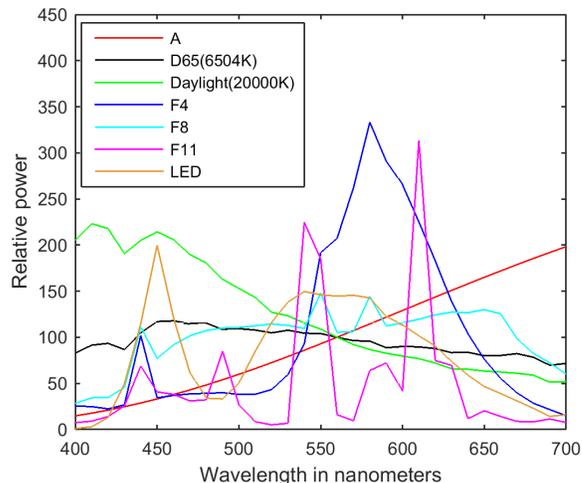
Figure 2: Spectral power distributions of the seven illuminants
