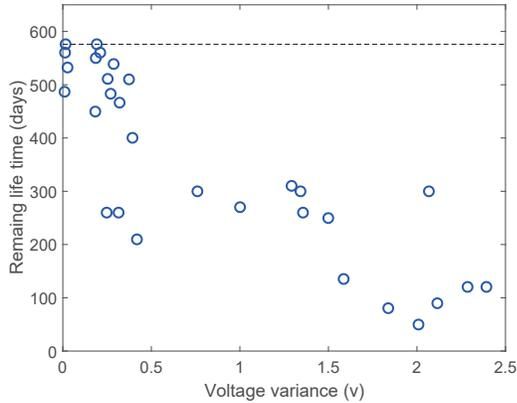
Figure 6: Correlation between the remaining life and voltage variance
