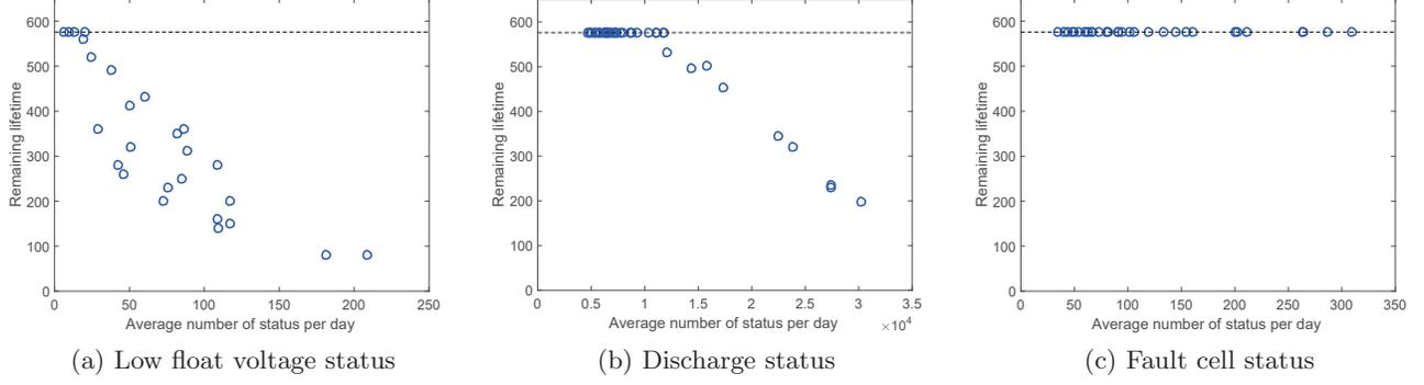
Figure 9: Correlation between the remaining life and the number of different status
