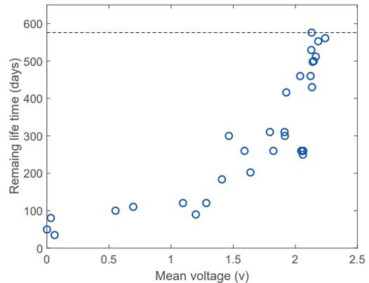
Figure 4: Correlation between the remaining life and mean voltage
