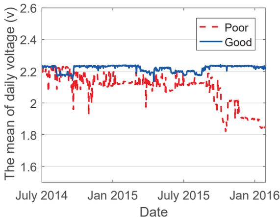
Figure 3: Mean voltage versus battery status
