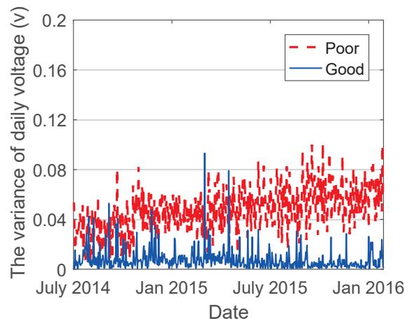
Figure 5: Voltage variances versus battery status
