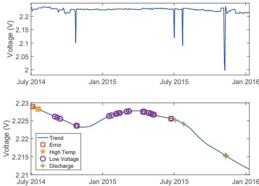
Figure 7: Example of time series showing battery aging phenomenon with status
