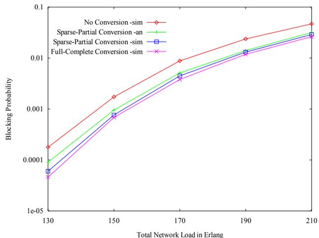
Fig. 8. Blocking Performance in NSFNET,  $M = 50$
