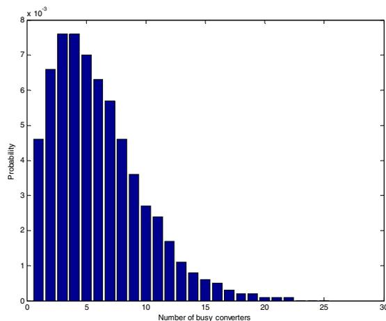
Fig. 7. Distribution of the number of busy wavelength converters at Node 4
