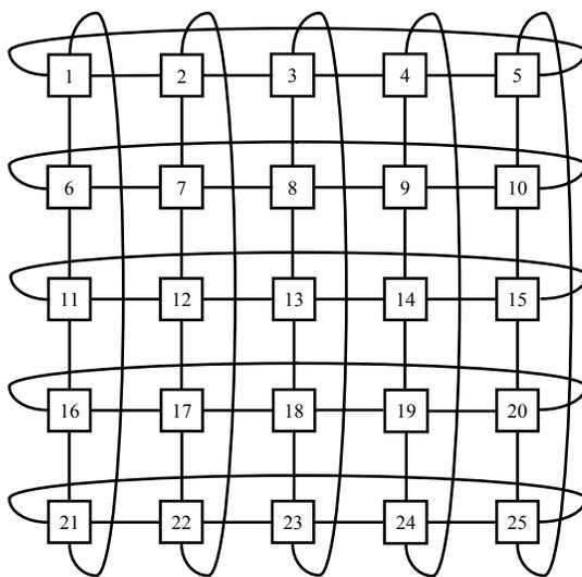
Fig. 9. 25-node Mesh-torus network
