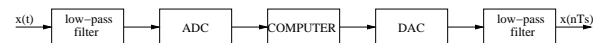
Figure 3: Low-pass filters in a digital audio system ensure that signals are bandlimited.
