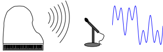
Figure 1: An analog electrical signal represents the pressure variations of a sound wave.
