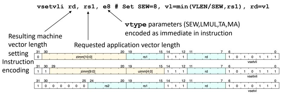
Usually use register-immediate form, **vsetvli**, to set **vtype** parameters. Immediate-immediate form, **vsetivli**, used when vector length known statically The register-register version **vsetvl** is usually used only for context save/restore
