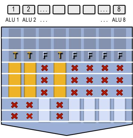
Not All ALUs do useful work Worst case: 1/8 peak performance Assume logic below is to be executed for each element in input array 'A' producing output into array 'result'
