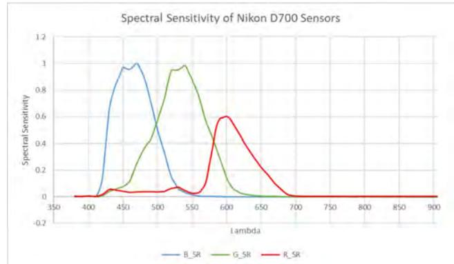
**Figure 1.** The spectral sensitivity functions of the Nikon D700 used in these experiments were generously measured by Image Engineering GmbH & Co. KG using their camSPECS device
