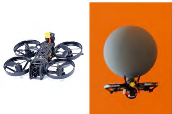
**Figure 3.** Right: CineBee 4K Whoop drone is used in the experiment to carry the grey ball around. The camera that comes with the drone is detached to reduce weight. Left: The drone carries the grey ball throughout each scene.
