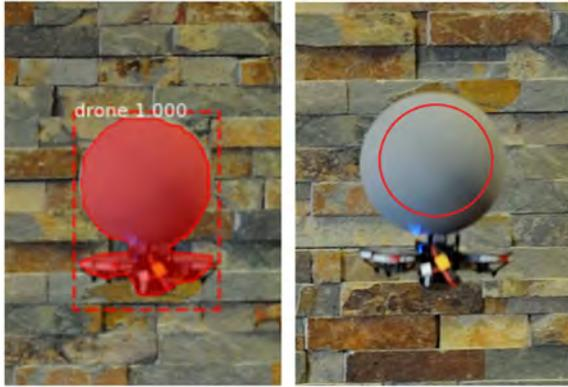
**Figure 4.** Left: The trained model detects the drone in the scene and then determines a bounding box and mask for the ball attached to a drone. The mask area is shown in red. Right: The red circle represents the area used for illumination colour measurement. The circle is detected using the Hough-circle transform in the given bounding box.
