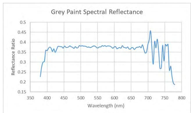
**Figure 2.** The spectral reflectance of Munsell Neutral 5 grey paint as measured from the painted ball using a SpectraScan PR650
