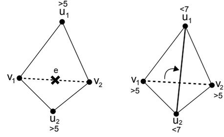
Figure 7: 5-6-7 preserving edge collapse (left) and edge flip (right).
