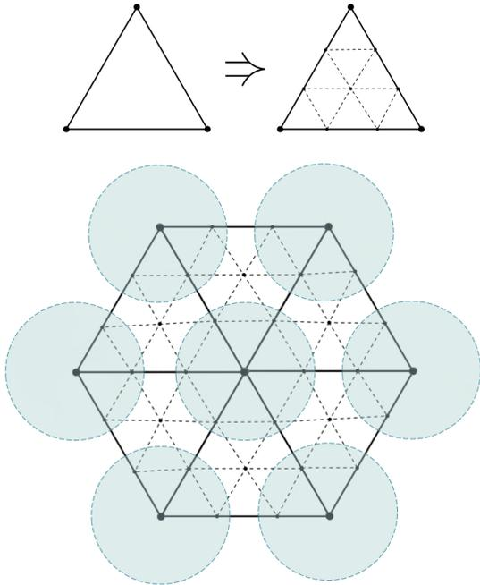
Figure 5: Topological subdivision to separate all the high-valence vertices sufficiently far apart from each other by at least two  $v_6$  vertices. The one-ring neighborhood that is not shared with other possible high valence vertices is indicated by the circles.
