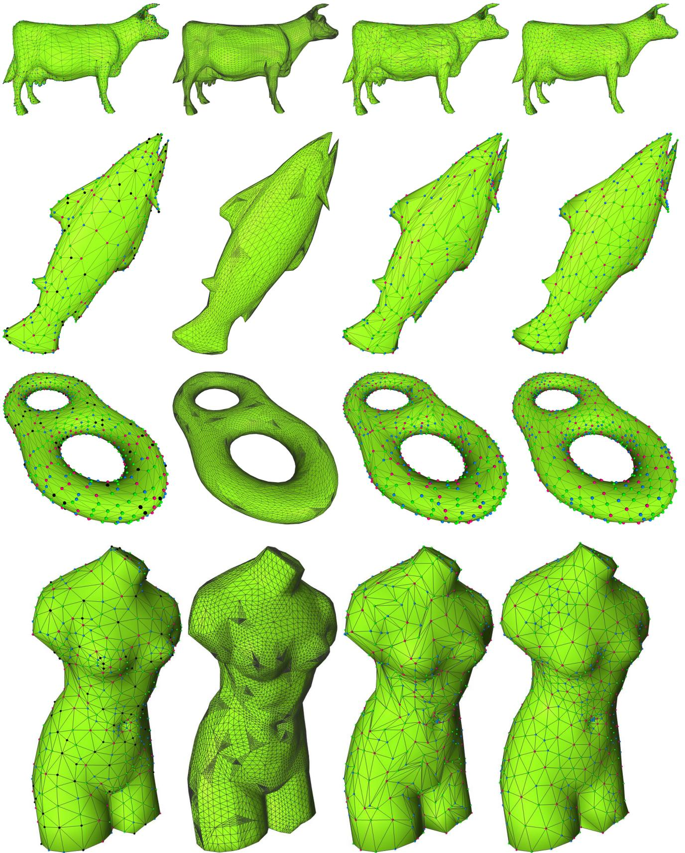
Figure 13: An example of feature preservation on a complex mesh(1st row), a mesh with fairly flat areas as well as some sharp feature regions(2nd row), a mesh with genus 2(3rd row), and the mesh of venus with subtle feature areas (4th row). From left to right: the original mesh, the 5-6-7 mesh, the decimated 5-6-7 mesh and finally the enhanced 5-6-7 mesh.
