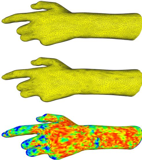
Figure 9: Visualization of Hausdorff distance error. Figures from top to bottom: the original mesh, the 5-6-7 mesh, the error visualization on the 5-6-7 mesh.
