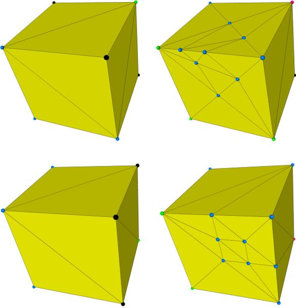
Figure 4: Demonstration of Valence 3(top) and Valence 4(bottom) removal on a cube.
