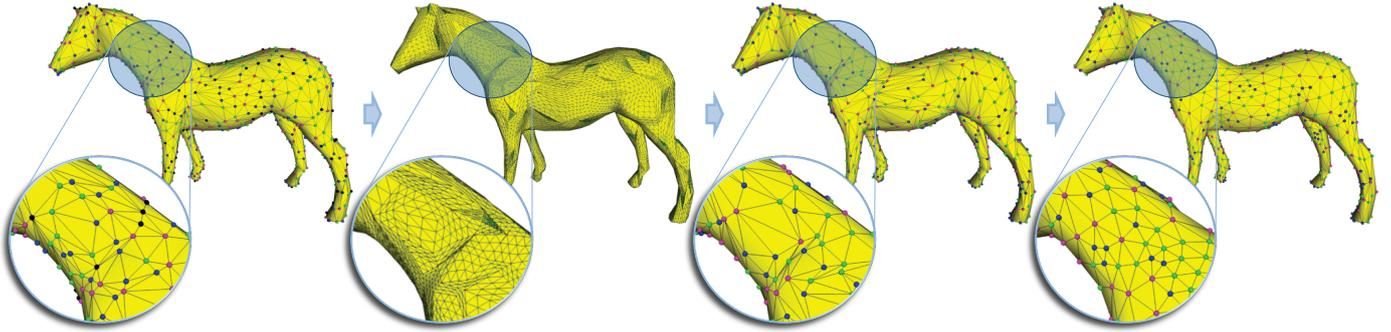
Figure 1: A triangle mesh (left) with low- and high-valence vertices (marked by black dots) remeshed into a 5-6-7 mesh with the same vertex count (right). Intermediate steps produce an initial 5-6-7 mesh (middle left) and a decimated version (middle right) which preserves the 5-6-7 property. The final mesh is produced with redistribution of vertices to improve sampling regularity, while respecting the features. Vertices of degrees 5, 6, and 7 are coloured by blue, green, and red, respectively.
