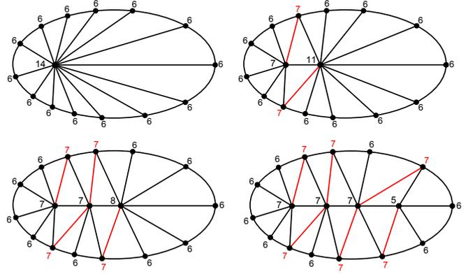
Figure 6: Elimination of a high-valence vertex ( $v_{14}$ ) by a series of vertex splits, where the ellipse denotes the one-ring neighbourhood of the vertex. This adds  $\lfloor \frac{14-2}{3} \rfloor - 1 = 3$  of  $v_7$  vertices and one  $v_{567}$  vertex (in this example, the  $v_5$  vertex in the bottom-right image), while increasing the valence of the neighbour vertices by at most one (i.e. from  $v_6$  to  $v_7$ ).
