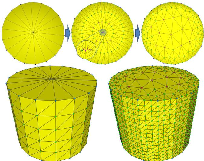
Figure 8: Comparison of the original cylinder mesh(left) with the 5-6-7 enhanced mesh(right). The top row from left to right: the original, 5-6-7, and 5-6-7 enhanced mesh (without decimation).
