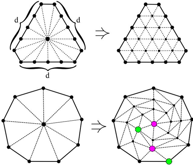
Figure 14: Two alternative schemes to remove a high valence vertex.
