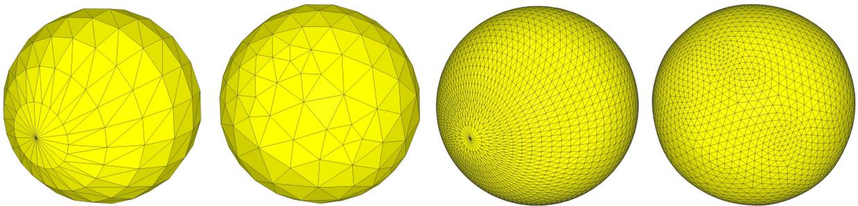
Figure 11: Results of subdivision on a sphere and the 5-6-7 sphere. Figures from left to right: 1) initial sphere 2) 5-6-7 sphere with the same vertex count 3) initial sphere after applying 2 steps of Loop subdivision 4) 5-6-7 sphere after applying 2 steps of Loop subdivision.
