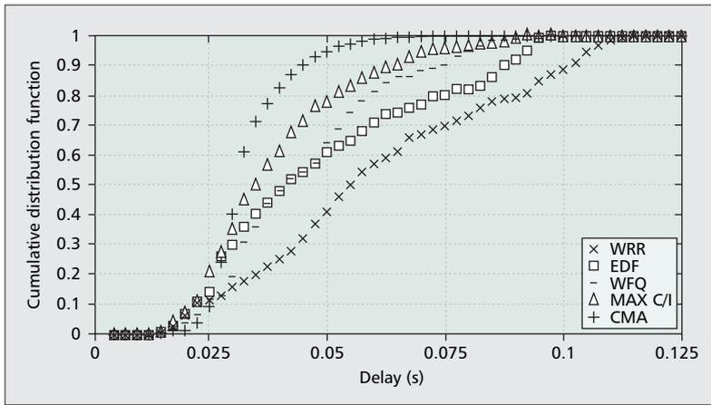
■ **Figure 5.** The 95th percentile CDF of E2E delay for rtPS services under different downlink scheduling schemes.
