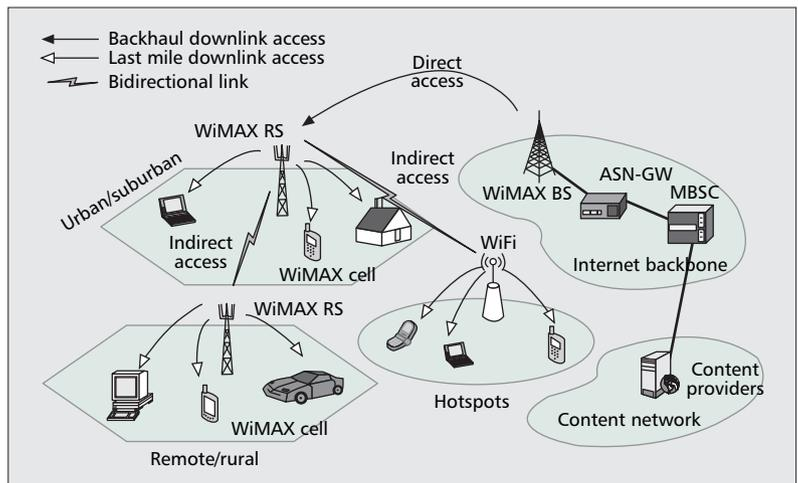
■ **Figure 1.** Multicast/broadcast WiMAX system architecture for MBS service delivery.
