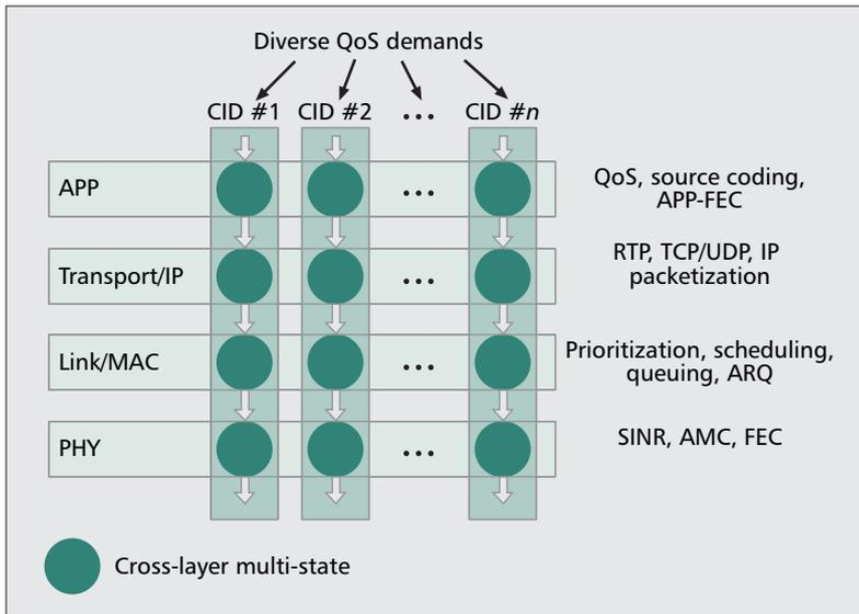
■ **Figure 3.** Connection-oriented multistate adaptation.
