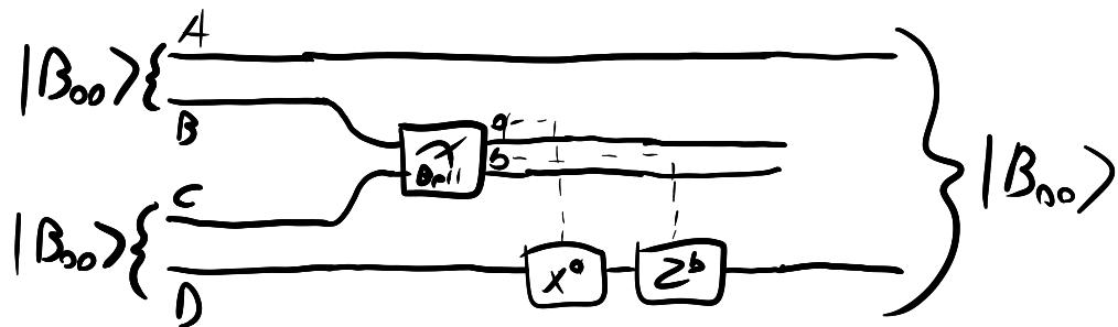
We can use this protocol to generate entangled pairs between any pair of **path-connected** processors, e.g.
