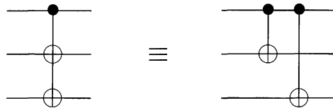
Figure 4.13. Controlled-NOT gate with multiple targets.
