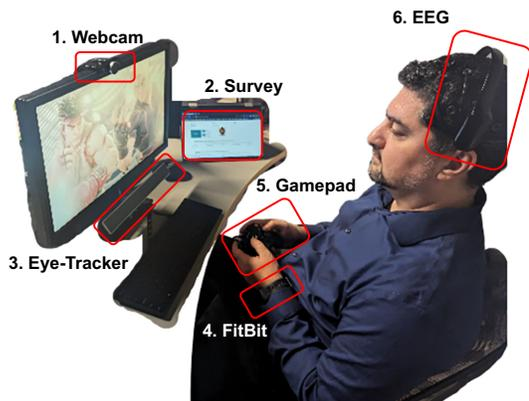
**FIG. 1. Experimental setup showing the integrated hardware components: 1) webcam; 2) survey tablet; 3) eye tracker; 4) smartwatch; 5) gamepad; and 6) EEG headset. ©ACM reused with permission from [8]/cropped and horizontally flipped from original and annotated.**
