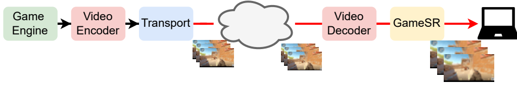
Fig. 1. GameSR in cloud gaming: low-resolution streams are rendered at server-side and upscaled at client-side in real-time.
