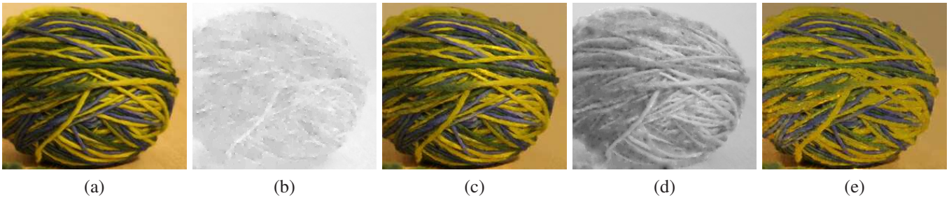
Figure 3. Ball of string. (a) Original image. (b)-(c) Shading and reflectance image without the use of texture cues. (d)-(e) Shading and reflectance image with our non-local texture algorithm.
