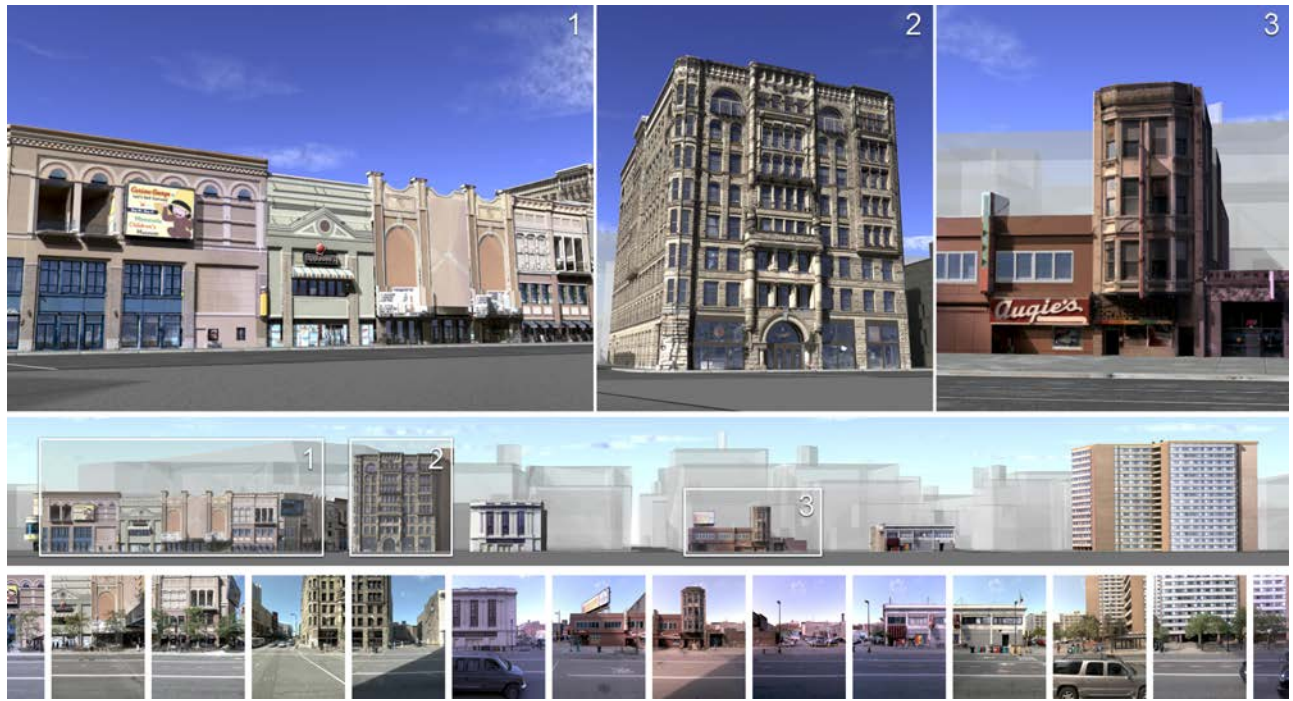
Figure 13: Modeling of Hennepin Avenue in Minneapolis from 281 images: some input images in the bottom row, the recovered model rendered in the middle row, and three zoomed sections of the recovered model rendered in the top row.
