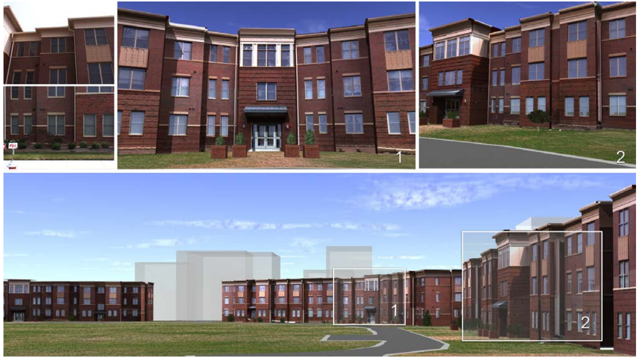
Figure 12: The modeling of a Chapel Hill street from 616 images (captured by UNC/UK) : two input images on the top left, the recovered model rendered in the bottom row, and two zoomed sections of the recovered model rendered in the middle and on the right of the top row.
